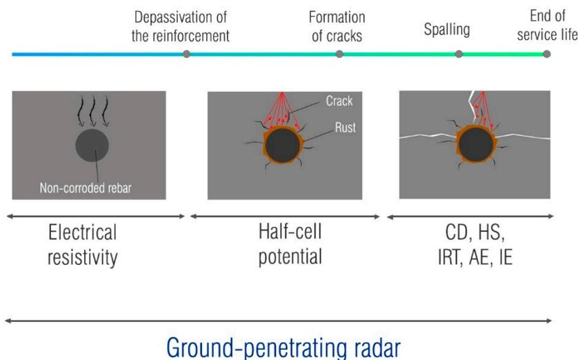
**Figure 5.** Multiple NDT used for the condition assessment.
