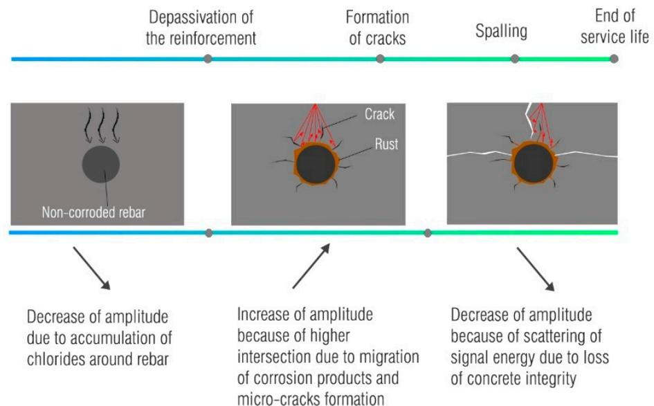
**Figure 3.** Changes in the GPR signal during corrosion process.
